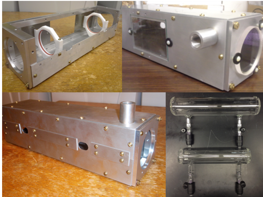
Figure 5.4: Photos of an optical pumping oven designed by the author, and a photo of two glass optical pumping cells, designed by colleagues of the author.
