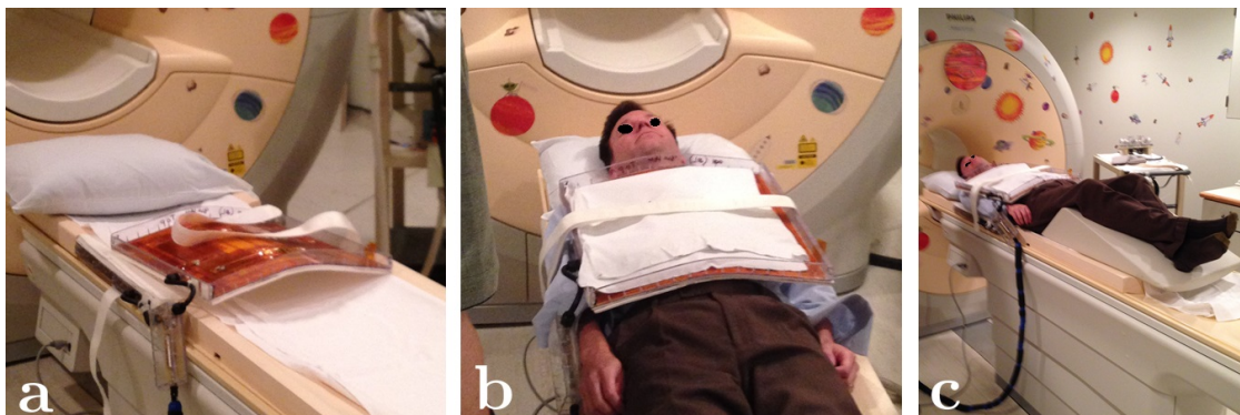
Figure 5.5: Photographs of the Multinuclear Coil and a Subject in the Magnet. Panel a: The ^{129}\text{Xe} coil (uncovered). Panel b: The coil placed on a subject (censored to conceal Jason's identity). Panel c: Subject with coil about to be placed in scanner bore.
