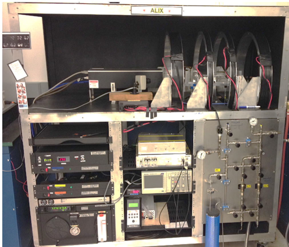
Figure 4.15: Photograph of the ^{129}\text{Xe} Polarizer 'Alix' designed and built by Laura L Walkup, Nara S Higano, and the author.
