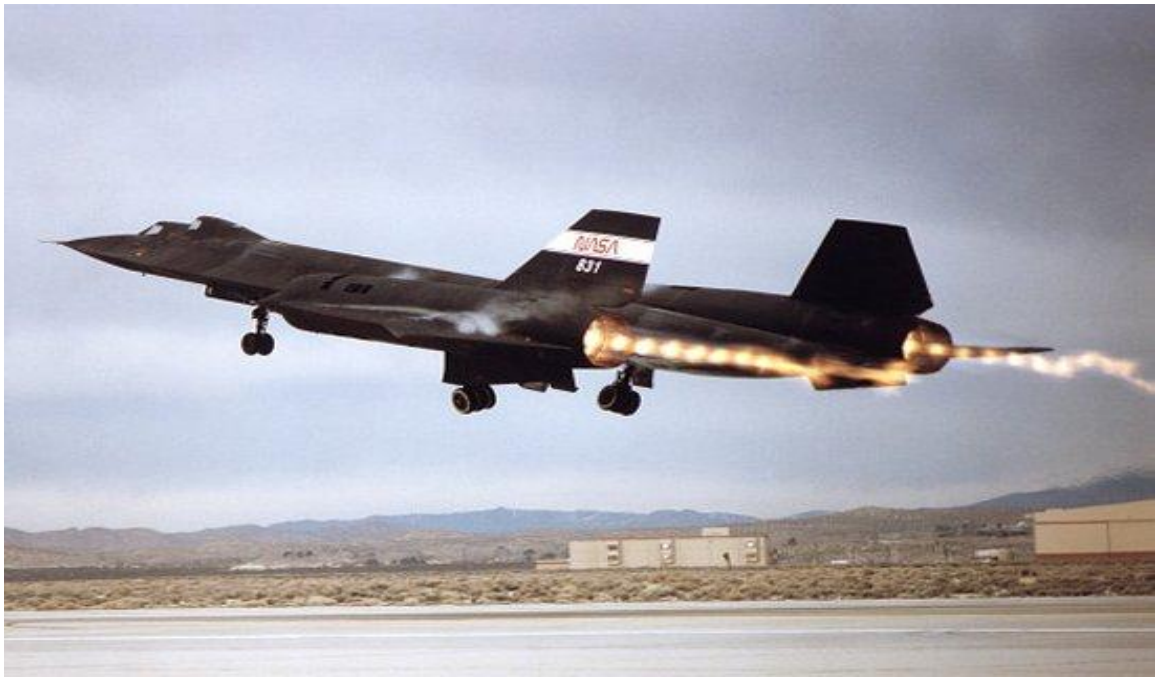
Figure 2.13: Shock diamonds in the jet engine exhaust of the SR-71 Blackbird during takeoff [12]
