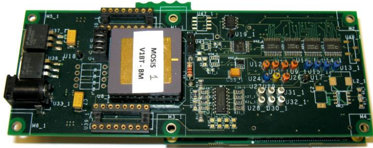
Figure 4.9: Custom printed circuit board (PCB) for testing and interfacing to the prototype test chip. The test chip is populated into a PGA65 socket on the board. On the bottom side, the PCB is connected to an FPGA board.
