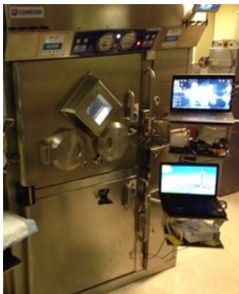
Figure 5.1. Examples of commercially available hot cell capable of housing and integrating with automated modules.
