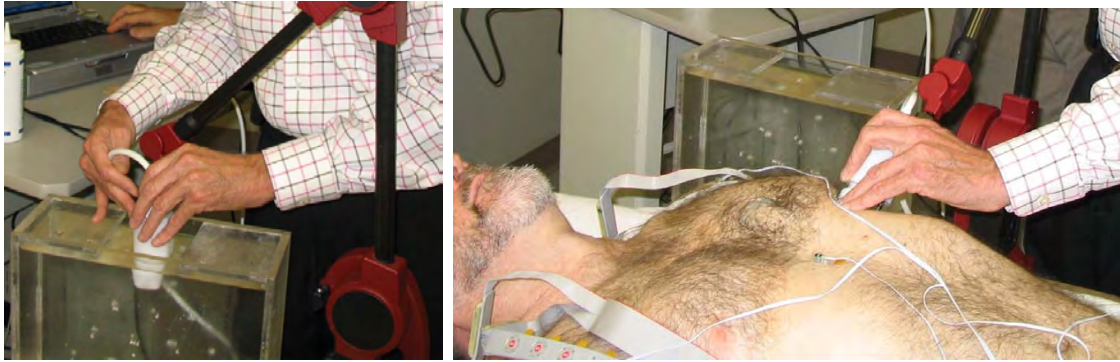
Figure D.1: Left) Calibration of the ultrasonic view plane with the custom phantom, Right) Ultrasonic scan of the heart with the Terason 3000 system using a 4VC (64-element, 2 MHz) transducer.
