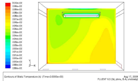
Figure 5.58 Temperature contours in yz-plane at z-50 after 5 minutes (vents open -flow on)
