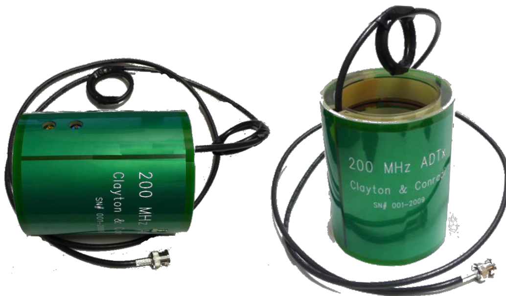
Figure C.3: The completed coil.
