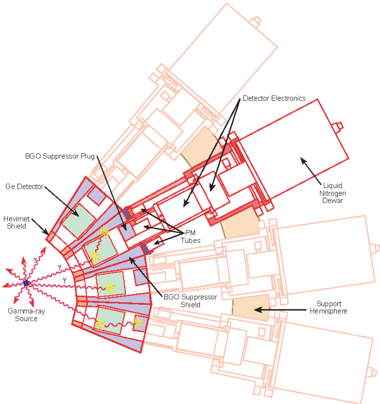
Figure 3-5: The modus operandi of Gammasphere. The HPGe detectors, their surrounding BGO Compton-suppression shields, hevimet shields, electronics, liquid nitrogen cooling system, and the support structure for a so-called hemisphere are all displayed. The \gamma rays illustrate a photoelectric interaction where all of the \gamma -ray's energy is deposited in the HPGe crystal and two Compton-scattering interactions where the BGO shield acts as a suppressor.
