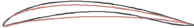
Figure 30: Comparison between the Optimized Hydrofoil Shapes for Deep Water and with Free Surface for V_\infty = 20 \text{ m/s} , Re_\infty = 20 \times 10^6 , \alpha = 6^\circ
