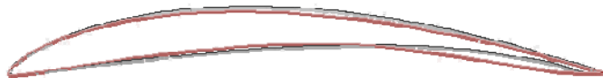
Figure 29: Comparison between the Optimized Hydrofoil Shapes for Deep Water and with Free Surface for V_\infty = 20 \text{ m/s} , Re_\infty = 20 \times 10^6 , \alpha = 4^\circ
