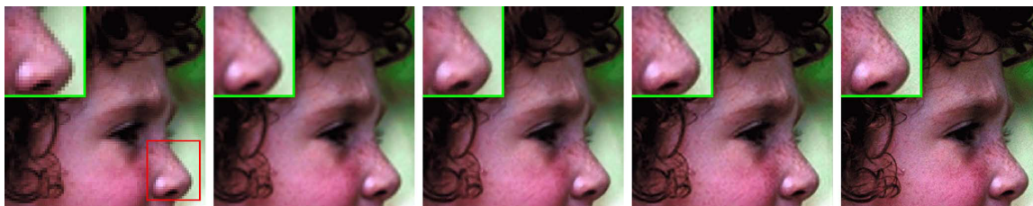
Figure 1.5: Single image superresolution results of the girl image magnified by a factor of 3 and the corresponding RMSEs. Left to right: input, bicubic interpolation (RMSE: 6.843), neighborhood embedding [2] (RMSE: 7.740), sparse representation [3] (RMSE: 6.525), and the original. (Reproduced from [3].)
