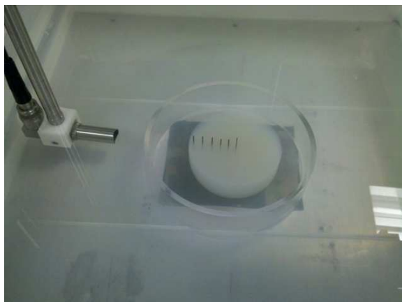
Figure 3.2: (Color online) A photograph of the pencil leads held in agar and surrounded by an acrylic cylindrical shell.
