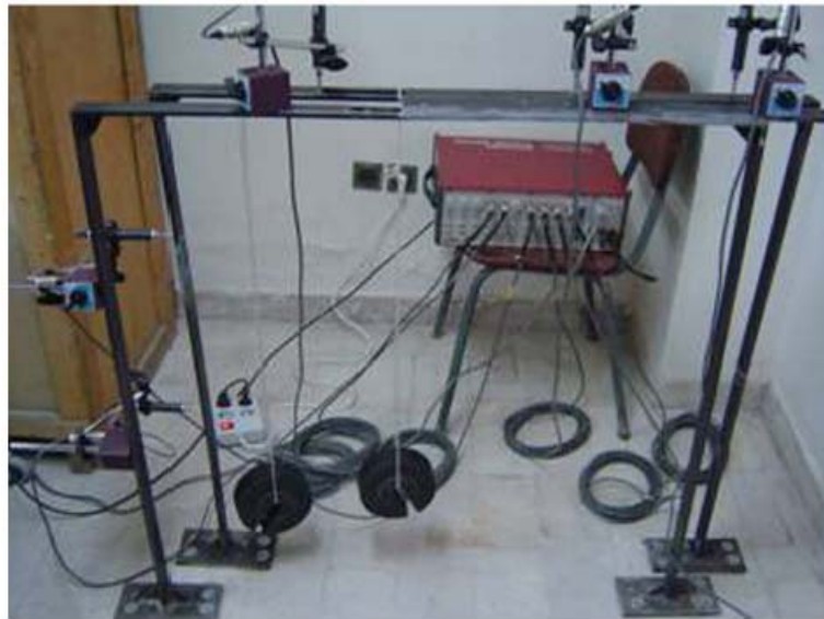
Figure 4.1 One Bay, One Story Steel Moment Frame Test Structure (reproduced from Bakhtiari-Nejad [2])
