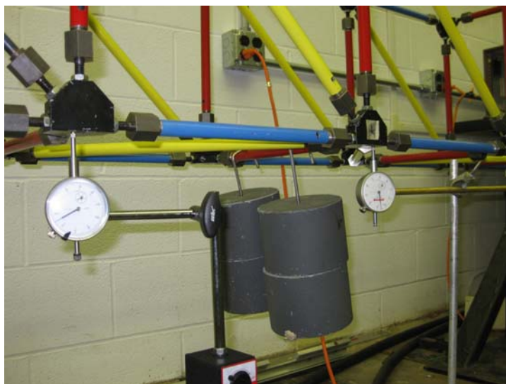
Figure 6.3 Typical Load Case Used for Damage Detection in Test Structure
