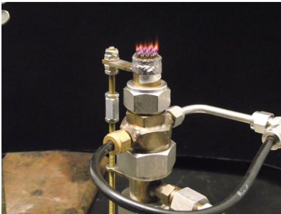
Figure 55 – Flame structure of the small scale microburner while producing cathode materials.
