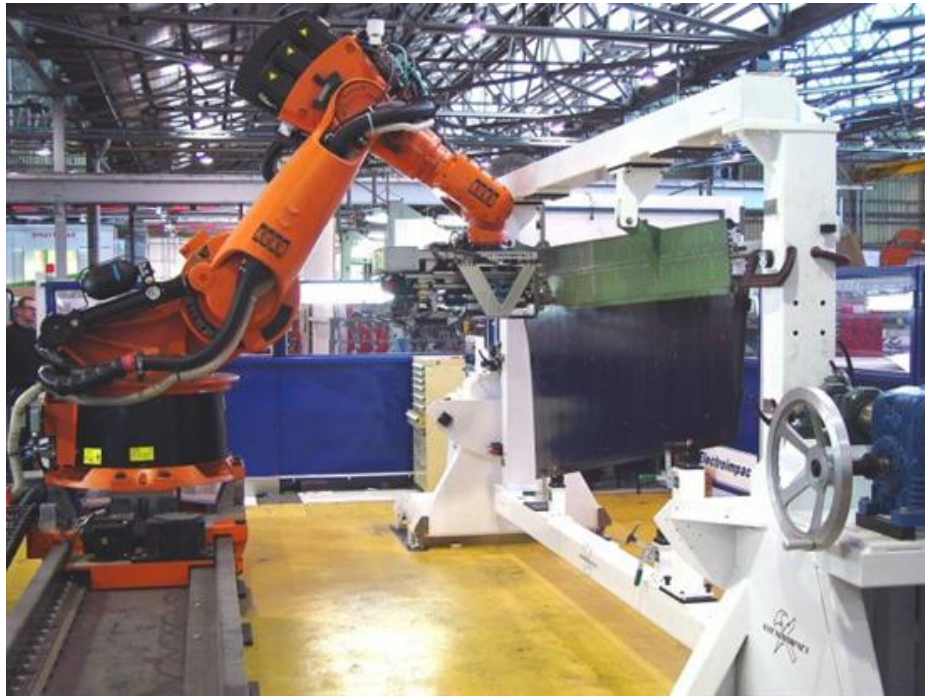
Figure 1.1: An example of a large scale aerospace drilling robot.
