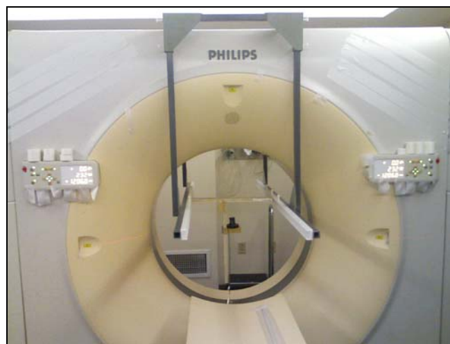
Figure 3.12 Fixture Holding the Solenoid Inside CT Bore
