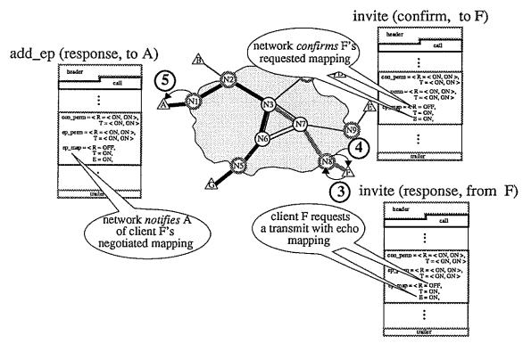
Figure 28. Invited Client Negotiating Connection Mapping (Continuation of Example from Figure 27).
