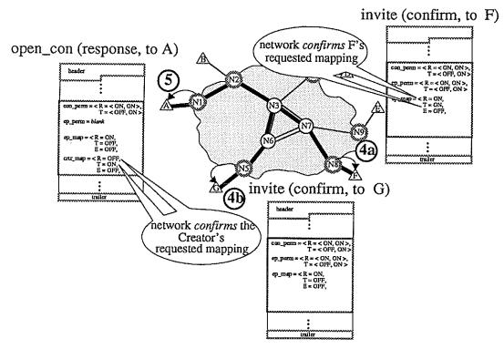
Figure 31. Invited Client Negotiating Connection Mapping (Continuation of Example from Figure 30).
