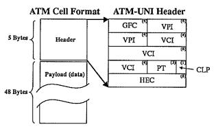
Figure 4. ATM UNI Cell Format.
