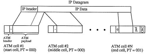
Figure 5. IP Segmentation/Reassembly Scheme.
