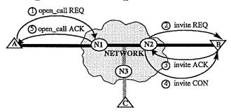
Figure 20. Building a Point-to-Point Call With One open call Operation.
