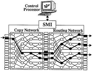
Figure 2. Architecture of Turner's Broadcast Packet Switch Demonstrating Multicast Routing.
