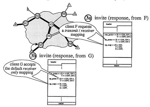
Figure 30. Invited Client Negotiating Connection Mapping (Continuation of Example from Figure 29).
