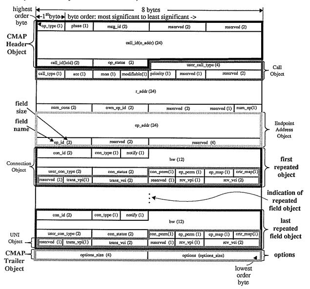
Figure 32. Common Message Format Characteristics (example open call(REQUEST))
