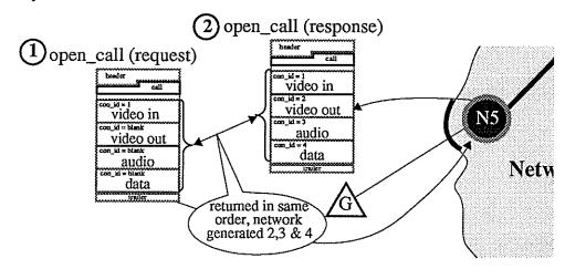
Figure 26. Mixing Client/Network Generated Connection Identifiers on open call Negotiation.
