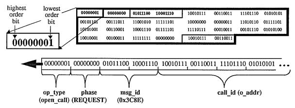
Figure 37. Byte/Bit Order of Transmission
