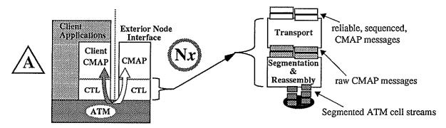
Figure 13. Client Access Protocol Stack for CMAP.
