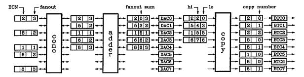
Figure 2: Example of Operation of Lee's Multicast Architecture
