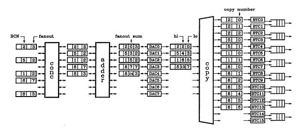
Figure 3: Example of System with Expanding Copy Network
