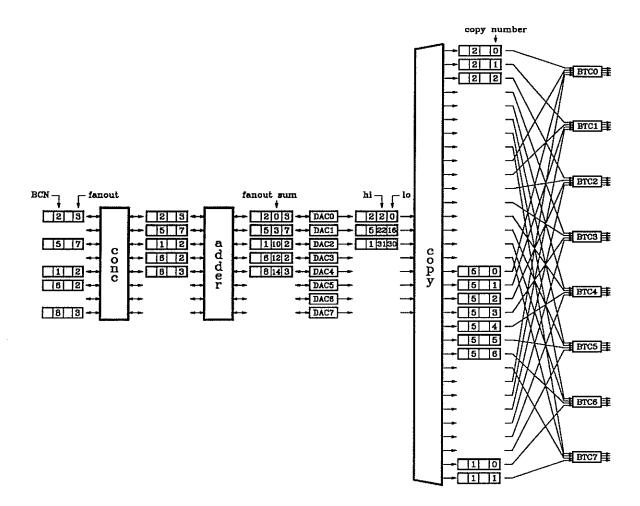
Figure 5: Copying with Fanout Aligned Addresses
