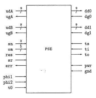
Figure 4.5: External Interface for Packet Switch Element Chip
