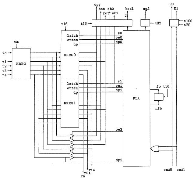
Figure 4.8: Input Control Circuit
