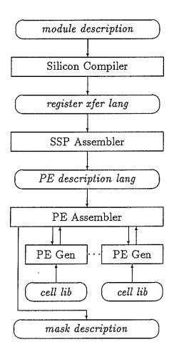
Figure 5.5: Structure of SSP Generator
