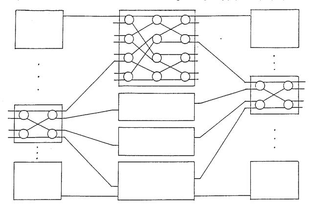
Figure 3.3: Construction of Delta Network with Distribution Stages
