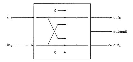
Figure 5.2: Unbuffered Switch Element
