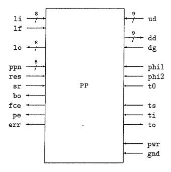
Figure 4.9: External Interface for Packet Processor
