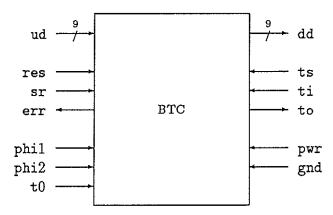
Figure 4.11: External Interface for BTC
