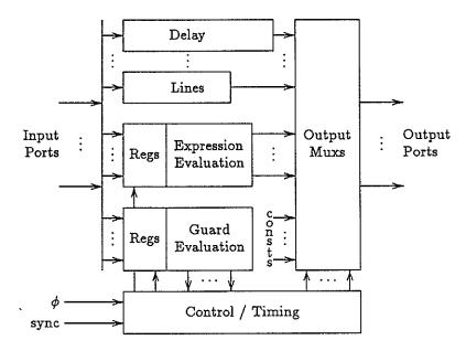
Figure 5.4: Target SSP Architecture
