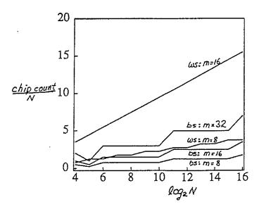
Figure 2.2: Complexity of Word-Serial and Bit-Sliced Benes Networks
