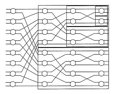
Figure 3.2: Recursive Construction of Delta Network
