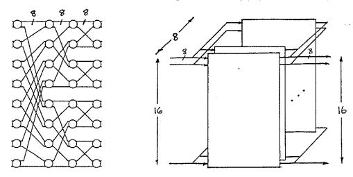
Figure 2.1: Word-Serial vs. Bit-Sliced Organization
