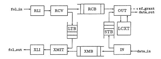
Figure 4.10: Packet Processor Circuit
