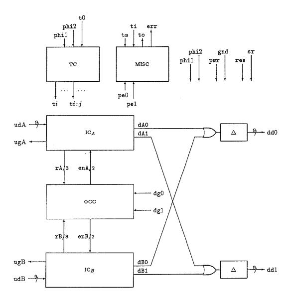
Figure 4.6: Block Diagram of Packet Switch Element Chip
