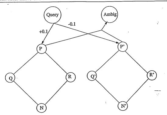
Figure 6: Inference engine for the Nixon diamond case: the two rings represents two similar subnetwork: One searches for a preferred model that satisfies the query and the other searches for a preferred model the falsifies the query.
