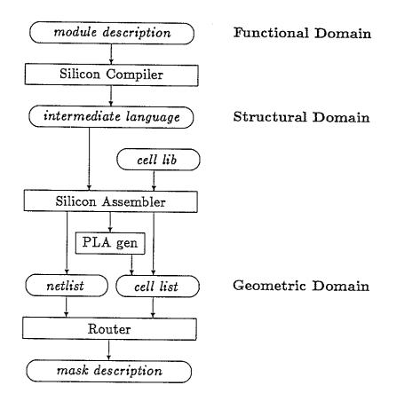
Figure 6.3: Structure of A Silicon Compiler
