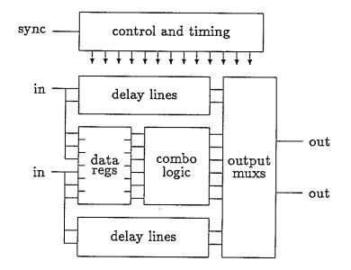
Figure 6.2: Target SSP Architecture
