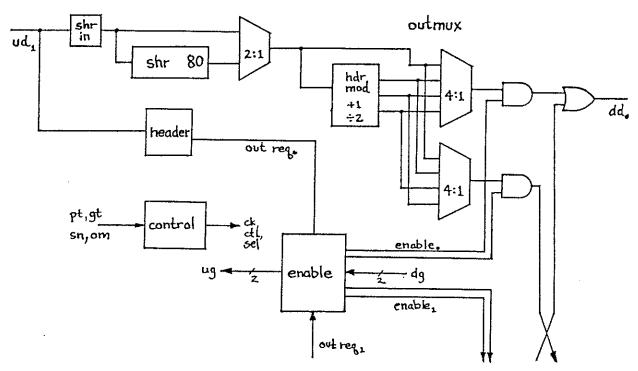
Figure 3.3: Block Diagram of Packet Switch Element Chip
