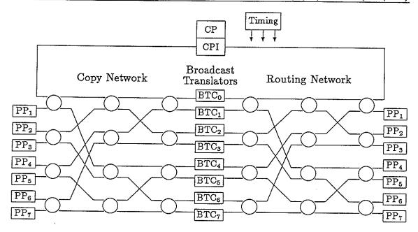
Figure 3.1: Prototype Switch Module
