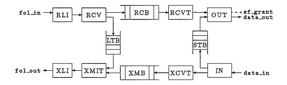
Figure 3.5: Packet Processor Circuit
