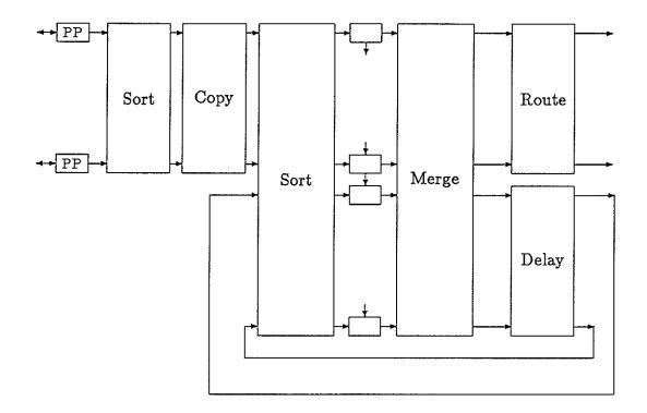
Figure 2.2: Starlite Switch Fabric
