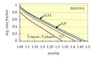
Figure 4. Miss fraction for DBL and BLOOFA on a variety of stress tests
