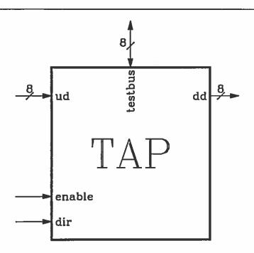
Figure 11. Interface Diagram for Tap
