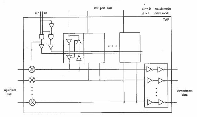
Figure 13. Block Diagram - Tap
