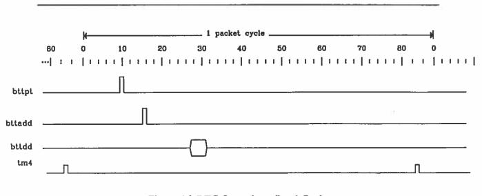
Figure 16. BTC Operation - Read Cycle
