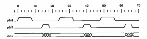
Figure 5. Clock and Data Relationship within a Clock Cycle
