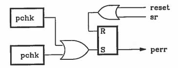
Figure 14. Block Diagram of Perr control circuitry.
