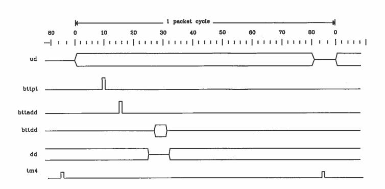
Figure 15. Global Timing of BTC for Broadcast Packet
