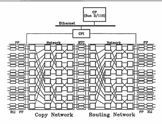
Figure 1. Switch Module
