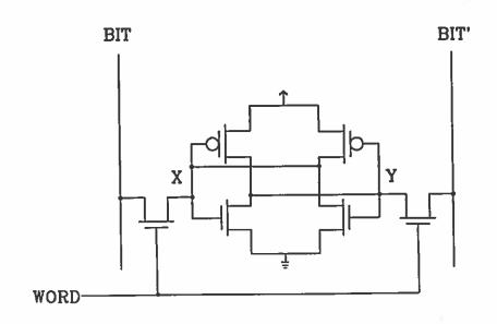
Figure 18. - 6 Transistor SRAM Cell
