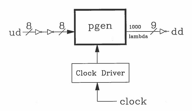
Figure 20. Parity generator Circuitry as simulated in FACTS
