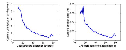
Figure 4: Errors vs. the orientation of the checkerboard plane
