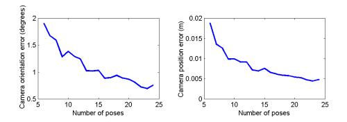
Figure 3: Errors vs. the number of poses of the checkerboard plane
