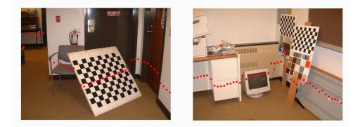
Figure 5: The left figure shows one checkerboard setting captured by the camera, and the red points overlaying on the image are the mapping laser reading with estimated extrinsic parameters  $\Phi$  and  $\Delta$ . The right figure shows one example of laser reading mapped onto the camera image after the extrinsic calibration
