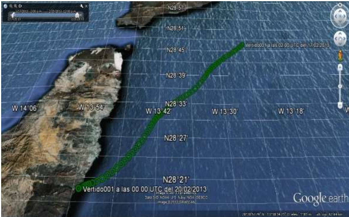
Figure 21: Path of the spill until it hits the coast of Fuerteventura. Region Canarias 6. TESEO Model.
