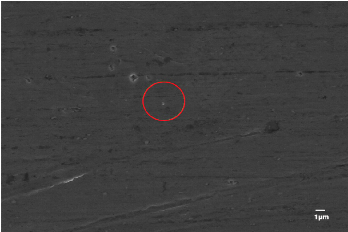
Figure 3. An example of a crater found on the interstellar collector. The crater is in the center of the red circle in the image.
