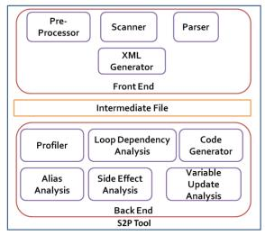
Figure 2: Block diagram of S2P tool.
