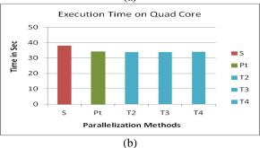
Fig.5. Execution timings of mp3 decoder on a file of size 6MB
