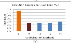
Fig.6. Execution timings of mp3 decoder on a file of size 27.7 MB
