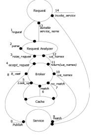
Figure 3 : Flow Diagram of web service discovery algorithm
