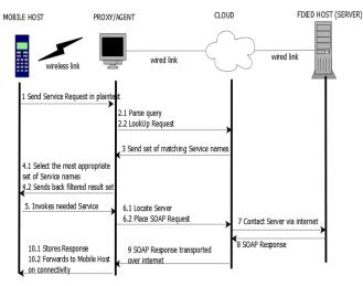
Figure 7: Locating needed services with modified x-SOA in mobile computing environment
