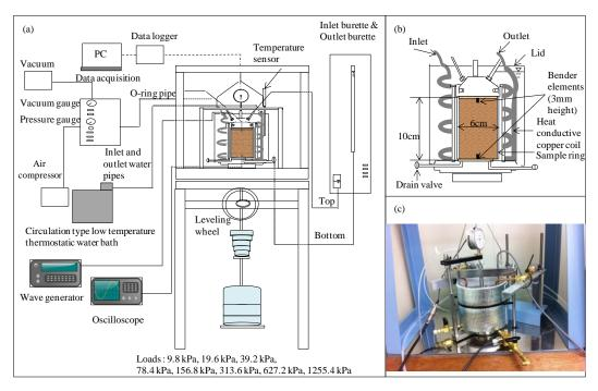
Fig. 1. (a) Overview of a modified oedometer apparatus (b) Detail of sample cell (c) Photo of sample cell
