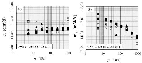
Fig. 3. (a) The coefficient of consolidation ( $c_v$ ) vs mean pressure (p) (b) the coefficient of volume compressibility ( $m_v$ ) vs mean pressure (p). Open symbols represent the results for  $\phi$  6m x H 10cm samples and filled symbols represent the results of  $\phi$  6m x H 2cm samples.
