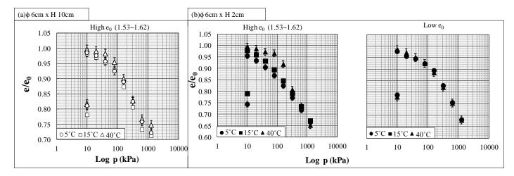
Fig. 4. Normalized e-Log p curves (a)  $\phi$  6cm x H 10cm samples (b)  $\phi$  6cm x H 2cm samples.
