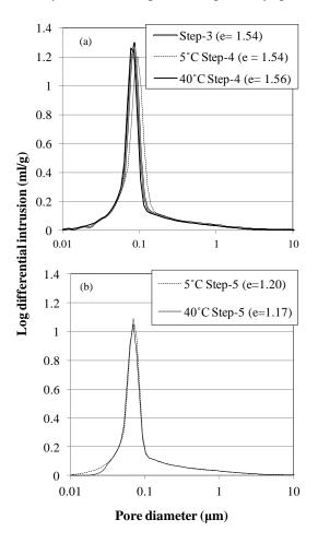
Fig. 8. Pore size distribution curves obtained using samples at experimental procedure Step-3 and Step-4 (Fig. 2), at 5 °C and 40 °C (b) Pore size distribution curves obtained using samples from Step-5, at 5°C and 40 °C.
