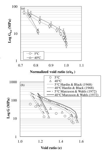
Fig. 6. The relationship between shear modulus ( $G_{b,e}$ ) and normalized void ratio ( $e/e_0$ ), obtained after 24 hours of each pressure (stress) step, at 5 °C and 40 °C (b) The relationship between measured shear modulus (G) and void ratio (e) as well as the estimated relationships using the Hardin & Black equation (1968) and Marcuson & Wahls equation (1972), at 5 °C and 40 °C.
