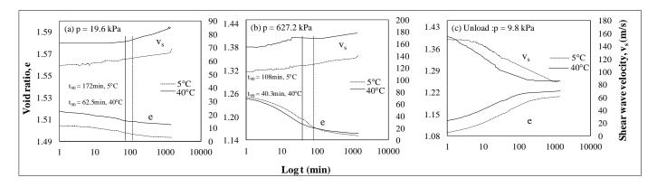
Fig. 5. An example of change of void ratio (e) and shear wave velocity ( $v_s$ ) with the logarithm of time (log t) at selected pressures (loading) (a, b), and at constant pressure of 9.81kPa (unloading) (c). The dotted lines show the data obtained at 5 °C and solid lines show the data obtained at 40°C. The vertical solid line shows the time for 90% completed consolidation ( $t_{50}$ ).
