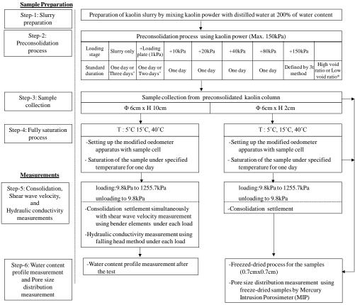
Fig. 2. The experimental procedures performed on the kaolin clay
