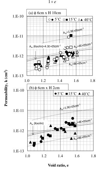
Fig. 7. The correlation between water permeability (k) and void ratio (e). The dotted lines are the predicted lines with respect to specific surface area  $(A_m)$  using the modified Kozeny-Carman equation. The solid line shows the predicted line using the measured specific surface area of kaolin clay. Open symbols represent the data obtained from direct measurement and filled symbols represent the data obtained by the modified oedometer using Terzaghi's theory of one-dimensional consolidation.
