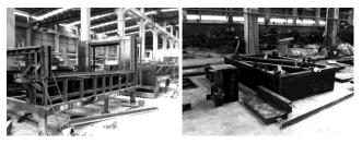
Fig. 14. Example of steel forms for mass production of precast façade elements
