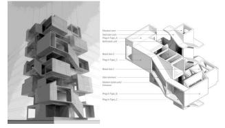
Fig. 12. *House me Tender* SML prototype and volumetric parts for a duplex unit.
