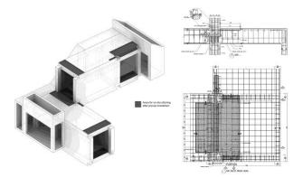
Fig. 16. Connection details between precast volumes.
