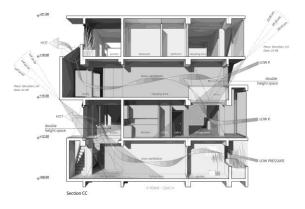
Fig. 15. SML prototype section showing environmental characteristics.
