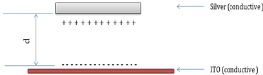
Figure.11: poles of the capacitor
