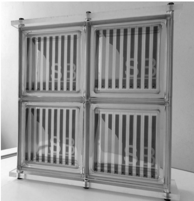
Figure 4. Prototype of dry-assembled DSC-integrated glassblocks
