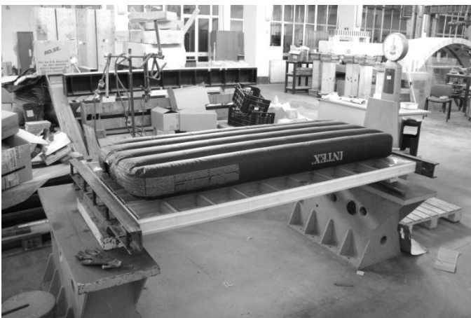
Figure 6. Laboratory load test on a 1.80 m 2 dry-assembled panel
