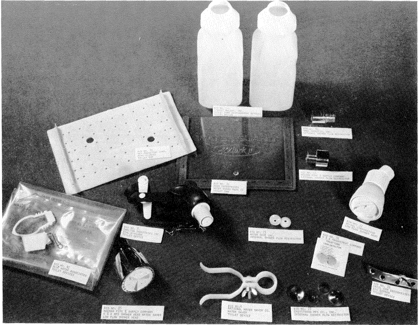
Many kinds of devices are available to help save water in toilets and showers. Dams, bottles, and bags reduce the amount of water used to flush a toilet; special shower heads and restrictors reduce shower flow. The Department of Water Resources tested 131 devices and selected 18 (13 are shown here) for use in the pilot program.
