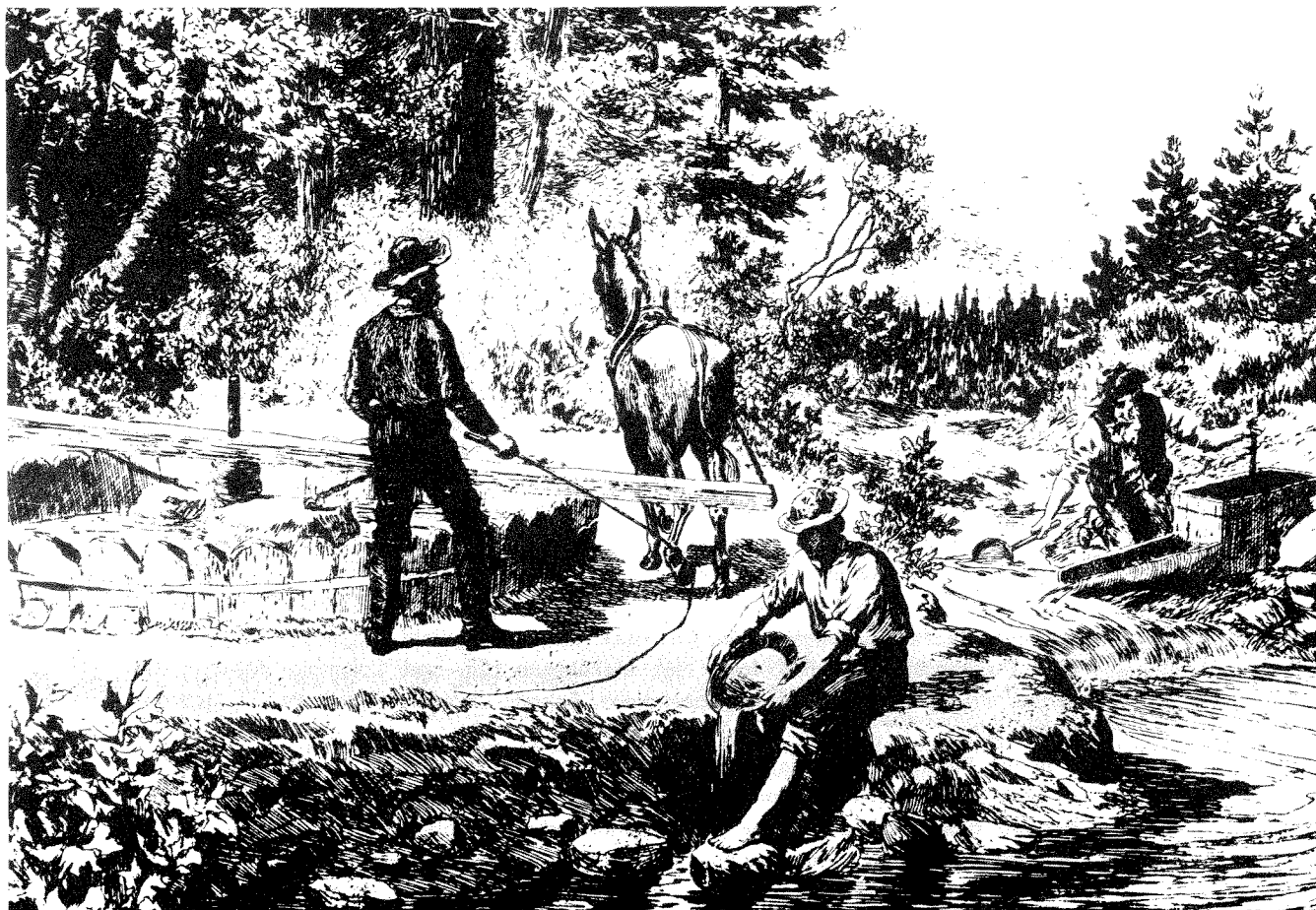
Photo 1. Early Gold-Mining Scene. One miner operates a horse-powered arrastra, a second pans ore and a third works with a rocker.
