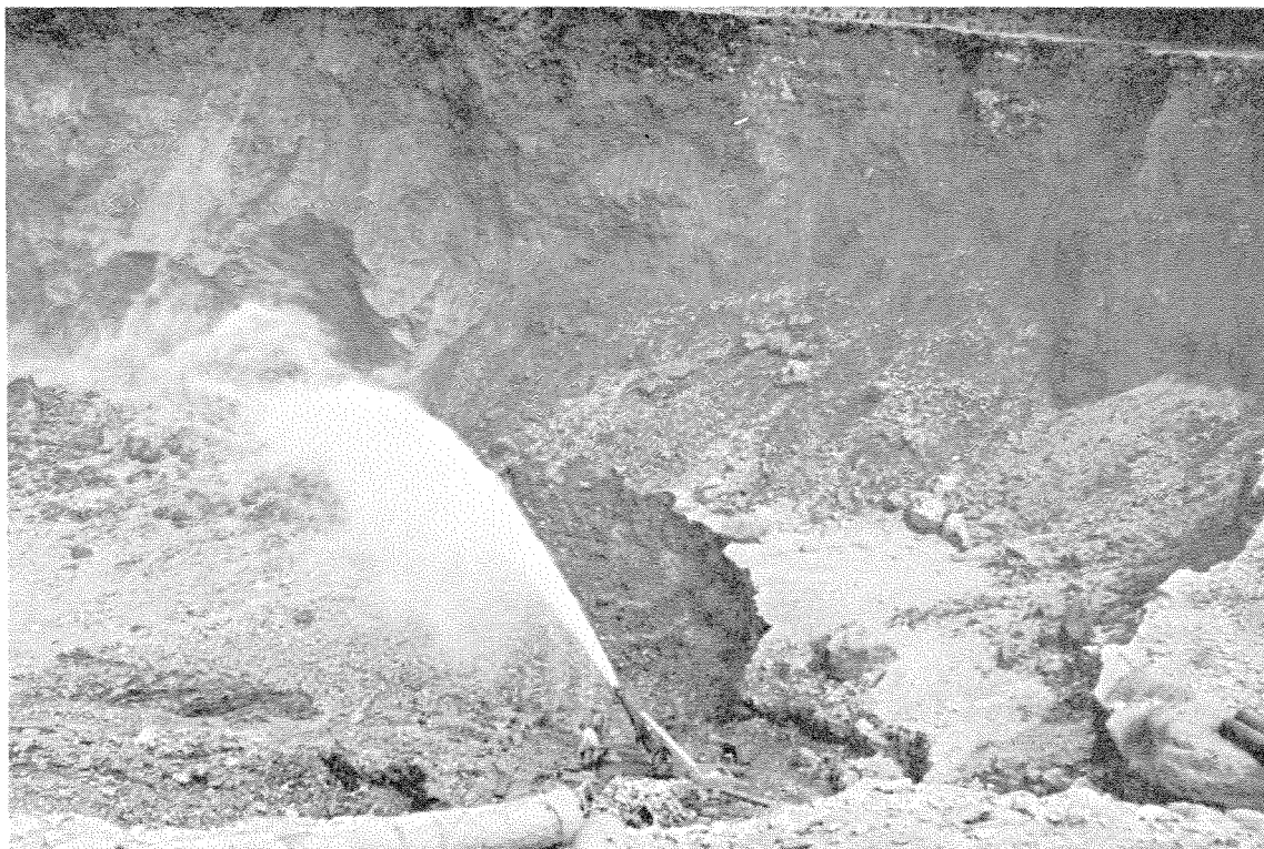
Photo 71. Hydraulic Mining of Bench Gravels, Trinity County. This is a 1933 scene at the Salyer mine. Photo by Olaf P. Jenkins.
