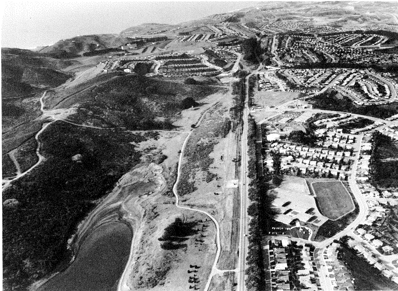
Photo 10. Urban development along the San Andreas fault zone south of San Francisco. The fault zone extends from sag pond in lower left of photo to upper center. Photo by Marshall Moxom.
