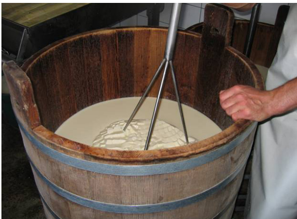
PHOTO 2. The « gerle » in action, with the beginning of decurding.
