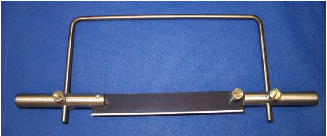
Figure A.5. Microtome blade attached to the holder device.
