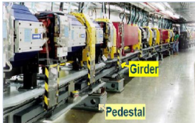
Figure 1.2: APS Steel box girders (Sharma, 2005)
