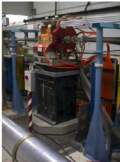
Figure 2. 23: FFTB Tunnel QC3 Magnet Quadrupole Anocast Stand (Fenn et al., 2004)
