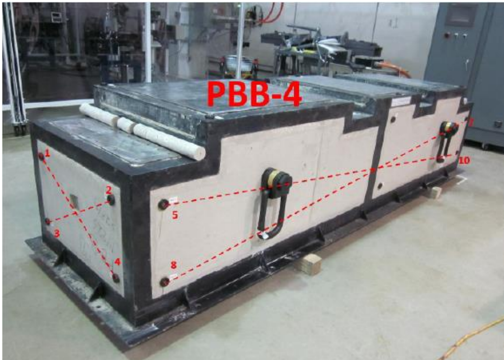
Figure 2. 28: Shrinkage Monitoring of Concrete Plinth Support (Collins et al., 2016)
