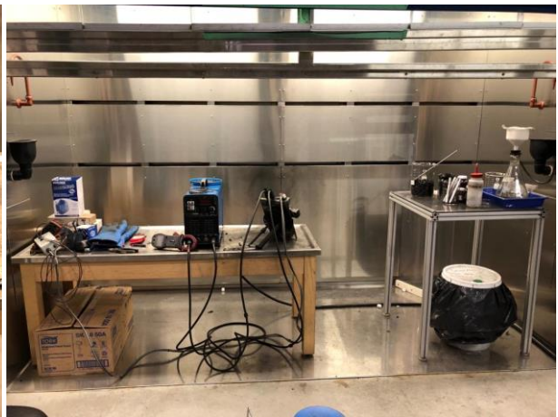
Figure A.1 Arc discharge setup and filtration area in the pilot plant.
