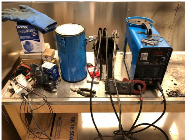
Figure A.1 Arc discharge setup and filtration area in the pilot plant.
