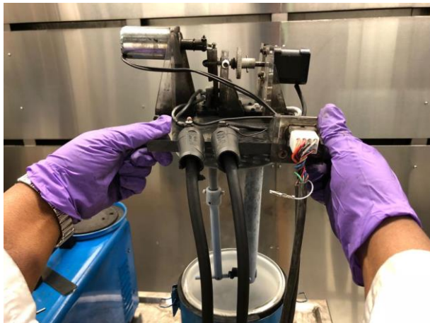
Figure A.2 Part of arc discharge setup showing mounted electrodes and some tools.
