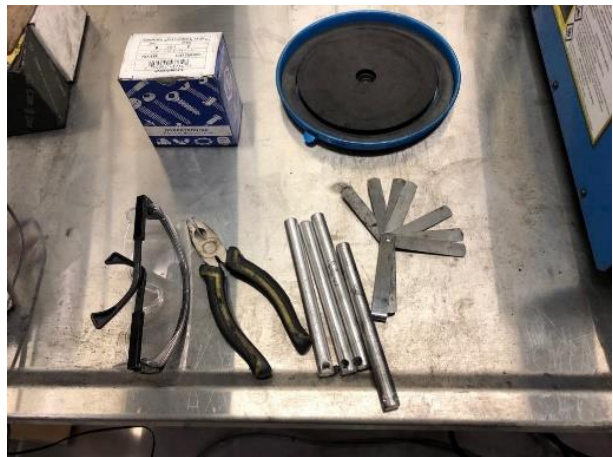
Figure A.2 Part of arc discharge setup showing mounted electrodes and some tools.
