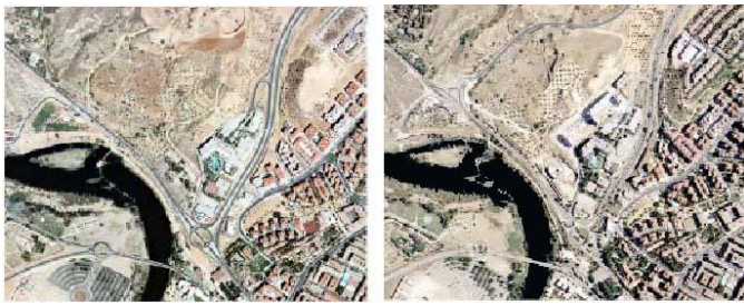
Fig. 5. Result of radiometric normalization. Reference image is on the left 1995, and normalized on the right 2005.
