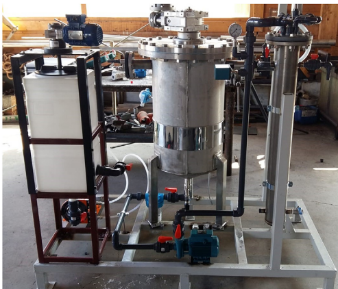
Fig. 3. Pilot scale anaerobic membrane bioreactor.
