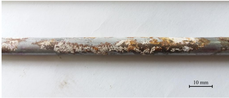
Figure 14. Uniform corrosion of uncracked sample after 168 days of exposure to 2% CO 2
