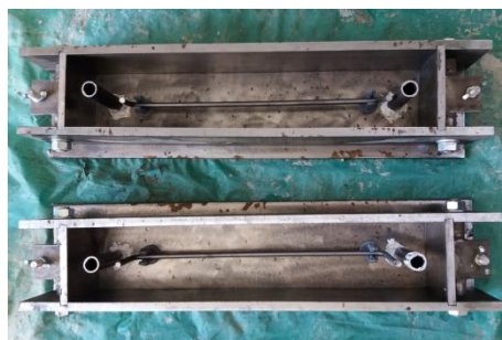
Figure 1. Preparation of the samples for the accelerated carbonation testing
