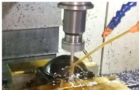
Gambar 4.26 Proses *Finishing* Kontur 2D
