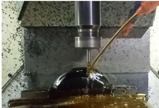
**Gambar 4.28 Proses *Finishing* Kontur 3D**
