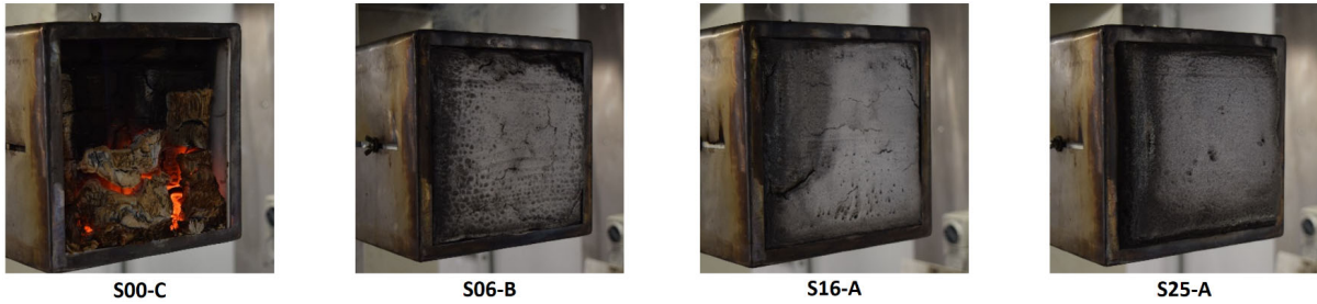
Figure 7. Comparison of uncoated and coated test samples at the end of fire testing.
