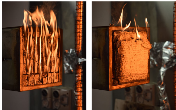
Figure 5. Flaming at the exposed surface of uncoated (S00-B) and coated (S06-A) samples during fire testing.
