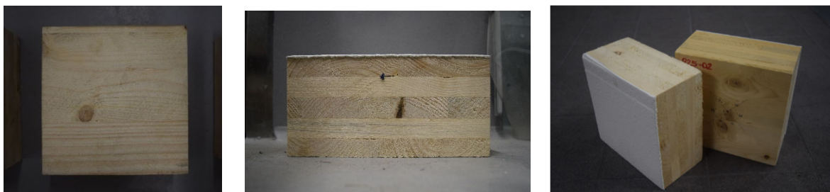
Figure 2. Uncoated and coated timber test samples.
