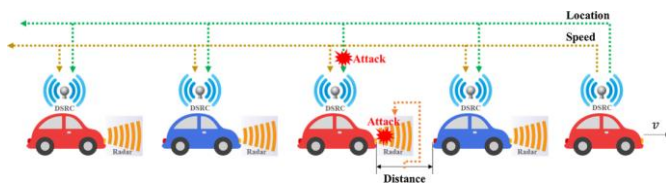
Figure 3. The operation of CCAV in platooning [20]
