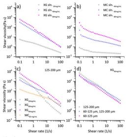
Fig. 4 Viscosity as a function of shear rate of (a) XG solutions (concentrations between 20 and 60 mg/mL), and (b) MC solutions (concentrations between 40 and 80 mg/mL) in DMEM; (c) Viscosity of pastes formed with CaP glass microspheres (0.48 g/mL of DMEM) of 125-200 µmm i DMEM with either XG or MC as an excipient; (d) Viscosity of microsphere pastes using different size range of CaP glass microspheres formed with 40 mg/mL of XG and DMEM solutions. All measurements were performed at 20 °C.
