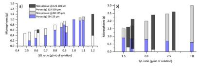
Fig. 8 Injectable formulations containing porous and non-porous CaP glass microspheres as a function of the S/L ratio (g/mL of solution); a) low S/L ratios (0.4-1.3 g/mL) obtained mainly through the combination of porous microspheres; b) high ratios (1.5-3.0 g/mL) obtained when
