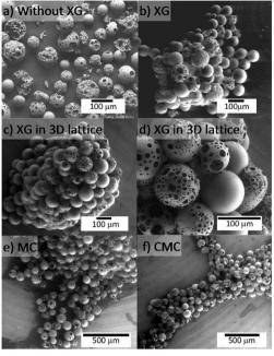
Fig. 3 Extruded pastes through a 3 mL syringe and 14G needle a) without XG; b) with XG; c) and d) with XG after testing into a 3D osteoporotic lattice (0.95 mm × 0.95 mm x 1.0 mm dimensions); e) Porous CaP glass microsphere pastes prepared with MC and d) with CMC. The images were collected in wet pastes without further preparation using an environmental SEM.
