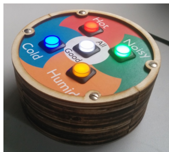
Figure 4: VoteBox , a system to collect subjective annotations on environmental data. The faceplate may be swapped out to update the categories under investigation, tailored to the individual concerns and needs of participants. As experiences of environmental (particularly thermal) comfort are inherently subjective, such a system provides a way of annotating how people actually feel, regardless of the sensed condition within the space.
