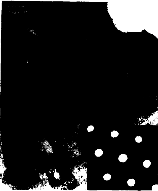
Fig. 4. Bright field TEM image of specimen 2. The diffraction pattern in the inset corresponds with a B[-111] orientation of the iron. The weak spots in the diffraction pattern are due to the long distance ordering of the nitrogen atoms in the interstitial positions of the pure iron lattice.
