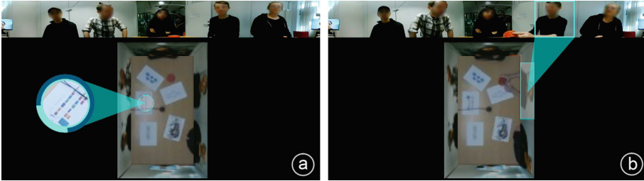
Fig. 3. GazeLens interface with (a) a lens showing a close-up of an artifact on the table and (b) a lens highlighting a hub worker’s position around the table. Lenses are triggered when users click on the video feeds, the lens on artifacts is rotated either by dragging the handle or simply clicking on the border at the desired direction.
