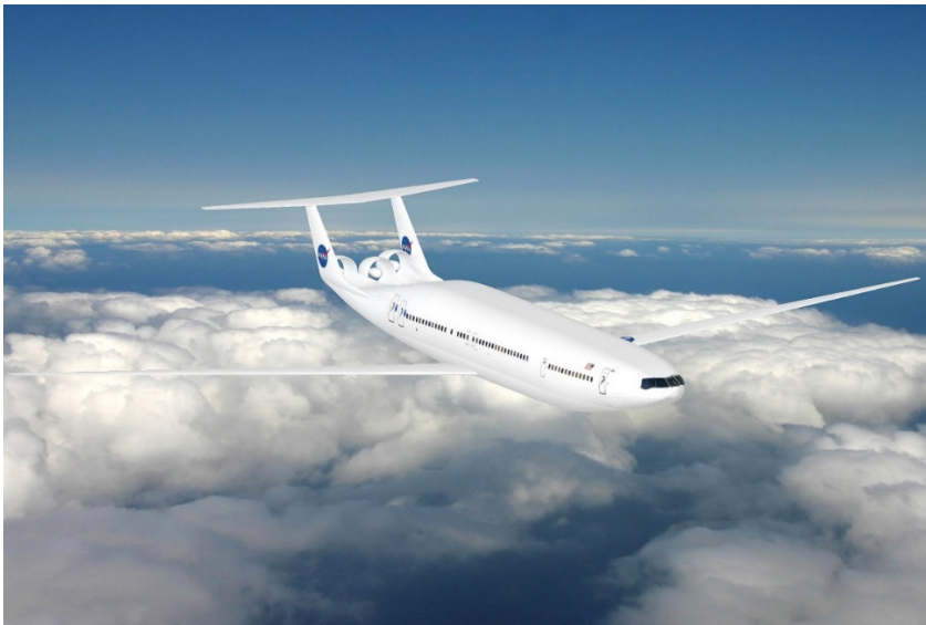
Fig. 10. The NASA/Aurora D8 ("Double bubble") aircraft concept [59].
